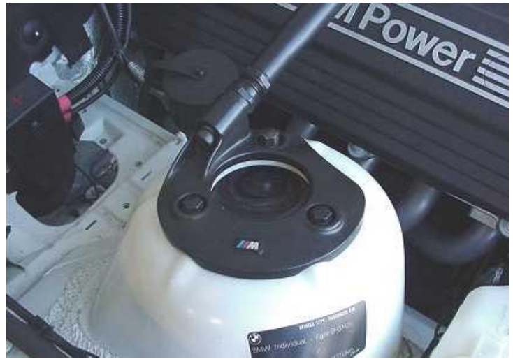
strut bar with moment connection and open tower cap
